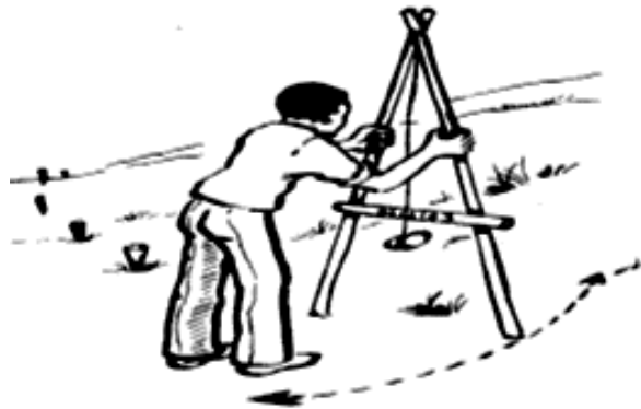
Figure 2.9: Marking grade lines with an A-frame
