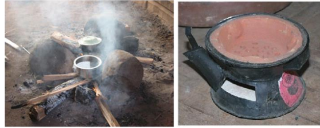
Fig 1. Traditional 3-stone open stoves and Lakech
