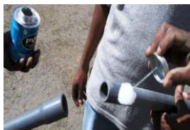
Figure 10.4 – Making the connection. Roughen up the inside of the female and the outside of the male part with sandpaper. Glue the pipes together. When glue the pipes together, only glue the male part. NOT the inside of the female part. If you do so, the male part will push the glue inside the female part forward, creating a rim on the inside, which could block the pistons.
