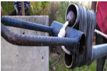
Figure 10.6 Guide Box with Rope and Pistons running through it
