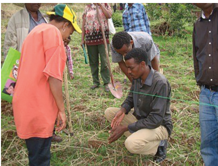
Figure 40: Field example of layout of a field using a line level (Ambo woreda, Oromia).
